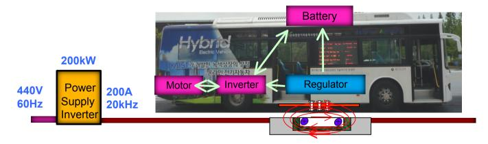
\* KAIST is demonstrating the core technology by using both power supply system under ground and power collection system attached to bus.
